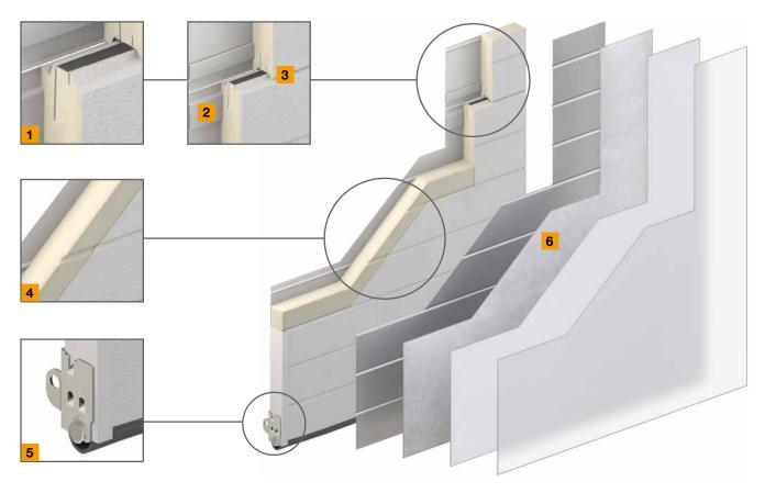
Precise Thermal Break 1 Increased thermal efficiency is achieved by our conductionresistant thermal break.
